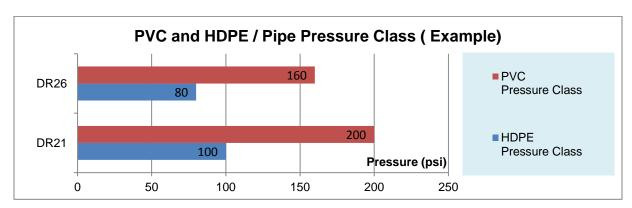
The designer cannot select which pipe (material) to use simply by specifying a pressure class (PC) for the application. There are pressure fluctuations in the system resulting from events such as pump start-up or shut-down and valves opening and closing.
