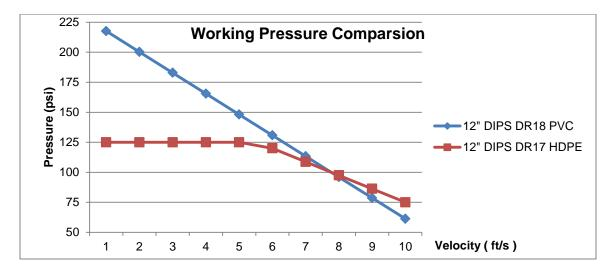
Below design velocity of 5.5 ft/s the working pressure is equal to the pressure class of HDPE (125 psi). Above the design velocity of 5.5 ft/s the working pressure is less than the pressure class of HDPE.
