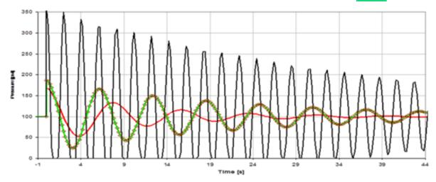
The pressure profile in a pipe due to dynamic system changes in flow velocity is so material property dependent, that there is no obvious simple way for pipes of different materials to have 'the same' pressure class. The difference in the ability of pipes of different materials to handle pressures caused by dynamic events means that PC alone cannot be the basis for the pipe selection.
