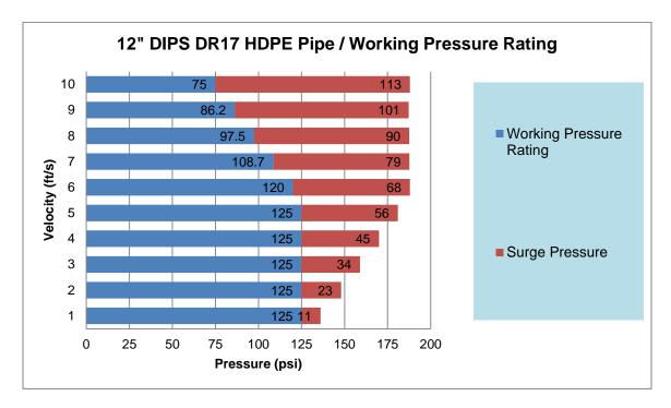
Stopping a flow that had a velocity of 5 fps will cause a pressure surge of 56 psi in a 12" DR 17 HDPE pipe. The anticipated pressure surge of 56 psi is less than the allowable surge allowance of 62.5 psi. The allowable working pressure of 125 psi need not be reduced since the surge pressure is less than allowable.
